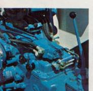
Auxiliary hydraulics. Single or double-spool remote hydraulic valves can be ordered factory installed on the 7000 tractor. Adds additional hydraulic versatility to your tractor.
