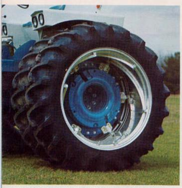
Dual wheels and big tires. For maximum traction and flotation, have your 7000 equipped with dual rear wheels or the new larger tires that are now available. The added traction and weight will more fully utilize the power of the 7000 tractor.
