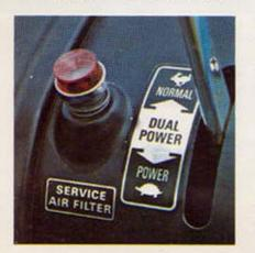
Dash-mounted warning light tells you when the air cleaner needs cleaning or service. Reduces need to check the filter element. Adds convenience, saves time.
