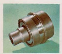
Here's the brain for the unique Ford Load Monitor system. This rugged mechanical device senses torque changes in the main drive line—and signals the hydraulic system to adjust working depth of the implement. Simple and strong—built to last and last... and last. Another better idea from Ford.
